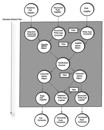
This diagram illustrates the event flow (upstream and downstream) within the notification communication model:
