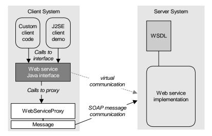
Figure 1: Interaction of J2SE client code with a Web service
