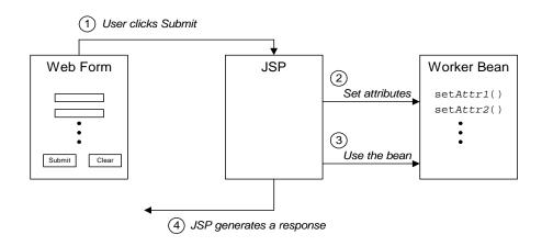
Figure 38: Processing Web Form Data Using a JSP
