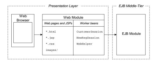
Figure 37: Overview of the J2EE Presentation Layer for AllDayBanking
