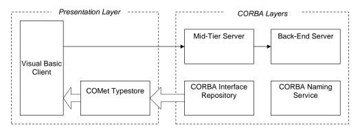
Figure 41: Architecture of the Visual Basic ATM Client Application
