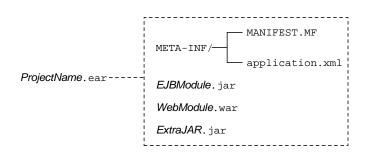
Figure 29: Standard Layout of an EAR File
