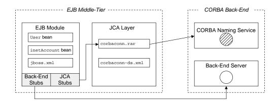
Figure 33: EJB to CORBA Connectivity Using Orbix Connect and JBoss
