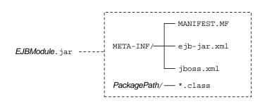
Figure 30: Layout of an EJB Module JAR File
