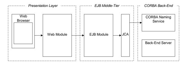
Figure 26: Architecture of the J2EE AllDayBanking Application
