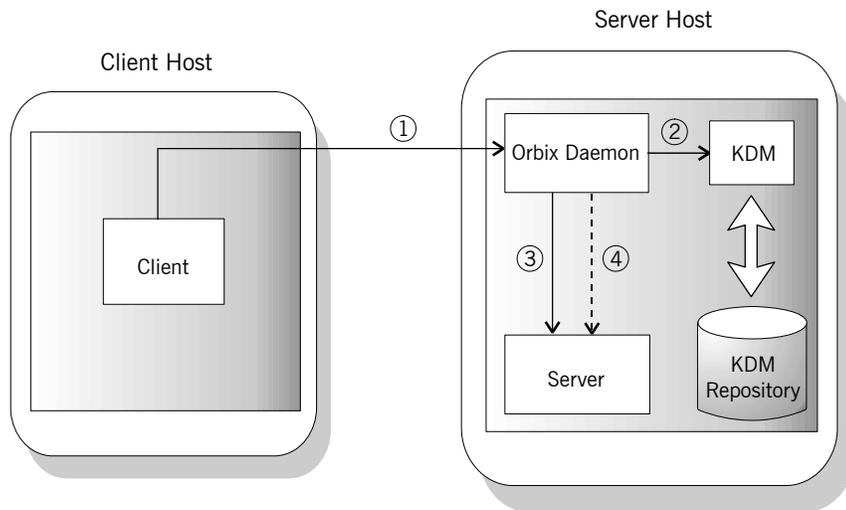
**Figure 4** Role of the Key Distribution Mechanism
