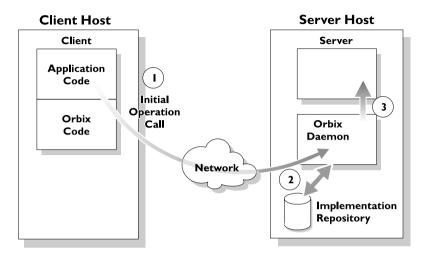
Figure 1.2: Automatic Launch of an Orbix Server Process
