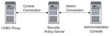
Fig. 1. Internal DBC communication links
