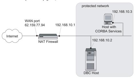
Fig. 2. The screened host firewall with I-DBC
