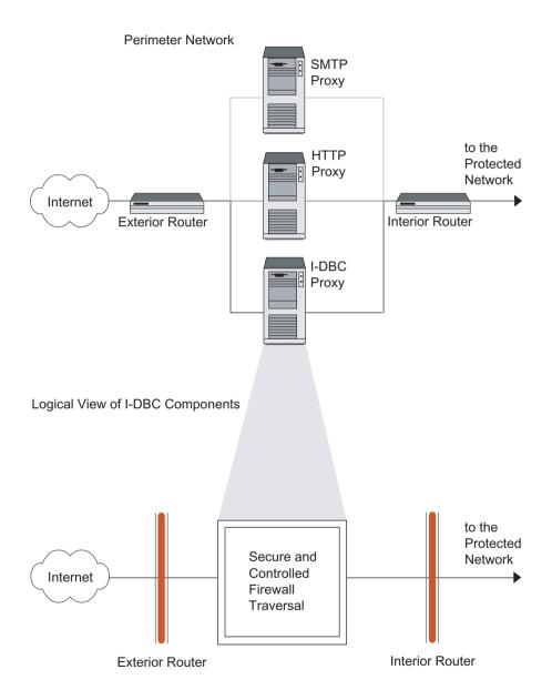
Fig. 2. I-DBC Components in a typical deployment Scenario
