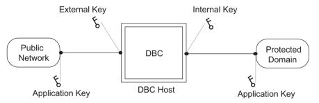
Fig. 63. Keys used on application connections
