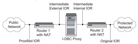
Fig. 5. Different types of IORs in a typical I-DBC Scenario
