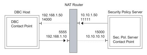
Fig. 57. NAT Router between the DBC Proxy host and the SPS host
