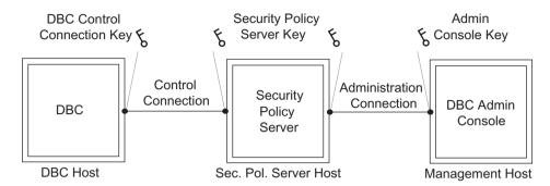
Fig. 64. Keys used on the Control and Administration Connection
