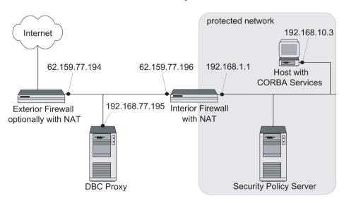
Fig. 3. Screened Subnet Firewall with I-DBC
