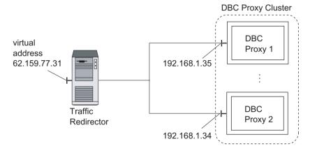
Fig. 31. External Interfaces and Virtual Address of DBC Proxies in a cluster
