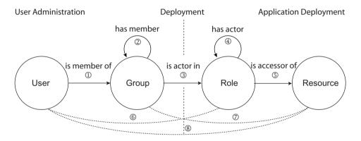
Fig. 1. Components of the access control policy
