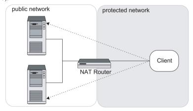
Fig. 7. Asymmetric NAT Mapping: The client is located in the protected network
