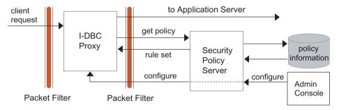
Fig. 1. Separation of I-DBC Components
