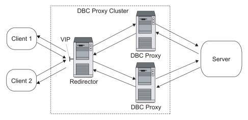
Fig. 10. Multiple I-DBC Proxies, balanced load
