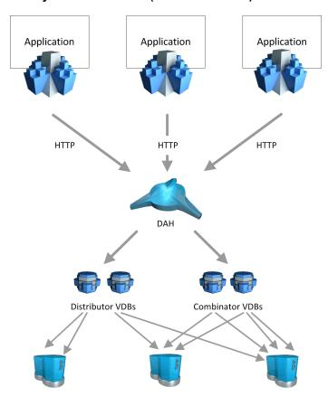
The DAH uses either combinator or distributor virtual databases (VDBs) to distribute the actions to one or more specific IDOL Server databases. The VDBs can map to one or more IDOL Server databases, or to other virtual databases that you set up for the DAH. The way a VDB forwards actions depends on its type.
