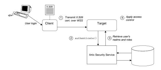
**Figure 13:** Overview of Certificate-Based Authentication with WSS
