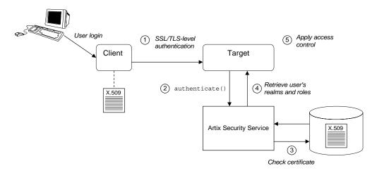
Figure 17: Overview of Certificate-Based Authentication
