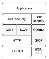
**Figure 9:** Example of an Application with Multiple Bindings
