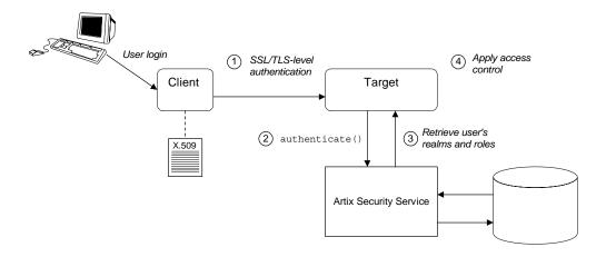
Figure 11: Overview of Certificate-Based Authentication with HTTPS
