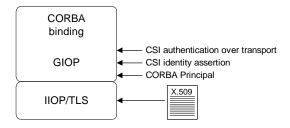
Figure 8: Protocol Layers in a CORBA Binding
