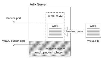
Figure 35: Endpoints Used by the WSDL Publishing Service
