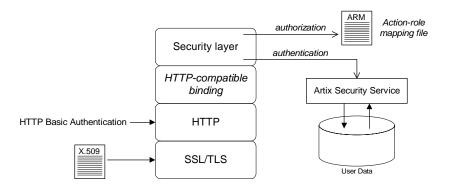
Figure 10: HTTP-Compatible Binding Security Layers
