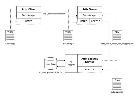
**Figure 4:** The Security Layer in the HelloWorld Example
