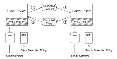
Figure 40: Basic Signing and Encryption Scenario
