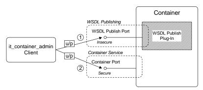
**Figure 5:** Connecting to a Secure Container Service
