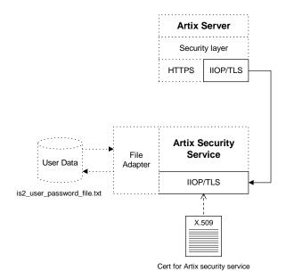
Figure 3: An IIOP/TLS Connection in the HelloWorld Example
