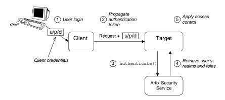
Figure 15: Two-Tier CORBA System Using CSI Credentials
