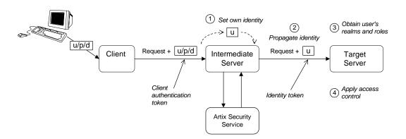
Figure 16: Three-Tier CORBA System Using CSIv2
