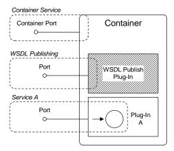
Figure 36: WSDL Publish Plug-In Deployed in a Secure Container
