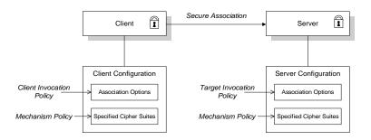
Figure 23: Configuration of a Secure Association
