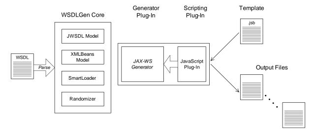
Figure 1: WSDLGen Code Generator Architecture
