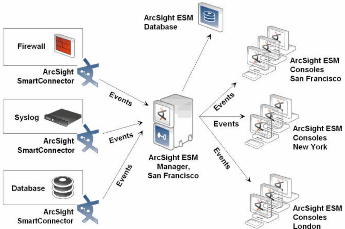
After the events are received by the Manager, it cross-correlates the events using rules, and sends meta-events to the database and to any Consoles that access the database.
