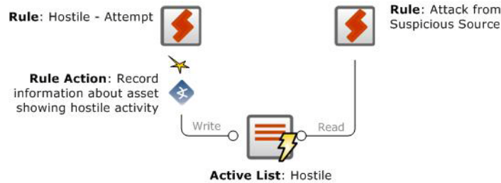
Figure 6-4 Using active lists to track data of interest. One rule can find an asset that shows hostile activity and write that asset's ID and activity information to an active list. Another rule can then read from the active list and take additional action, such as aggregate additional activity from that asset.
