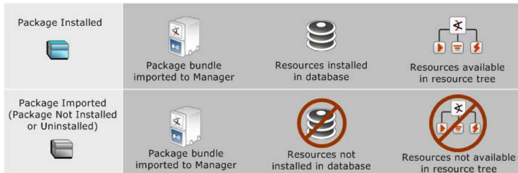
Figure 13-2 Packages imported and installed states. An installed package makes resources available in the resource tree. An imported package leaves the resources available in a zipped state on the Manager.
