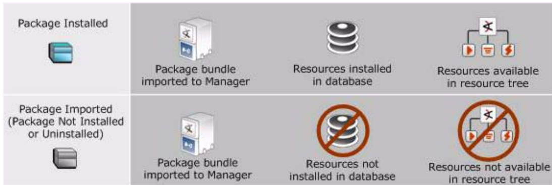
Figure 12-2 Packages Imported and Installed states. An installed package makes resources available in the resource tree. An imported package leaves the resources available in a zipped state on the Manager.
