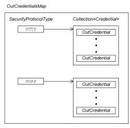
The OutCredentialsMap type is a map (of java.util.Map type) that associates each protocol key (for example, TLS, HTTP, or SOAP) with a collection of credentials. In this way, it is possible to associate one or more credential types with each layer of the transport protocol stack.
