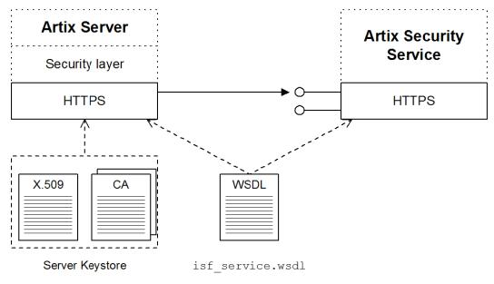
The server communicates with the security service using the SOAP binding and the HTTPS protocol. Connections to the security service are automatically opened by a security handler in the Artix server. First, the handler downloads the security service WSDL contract by querying the security service's WSDL publish port. Next, the handler connects to the Web services exposed by the security service, using the addresses from the downloaded WSDL contract.
