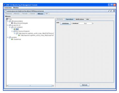
Figure 3: Managed Bus Operation in JConsole
