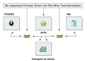
Because Artix ESB is built on top of ART, it is modular in nature. This means that it is highly configurable and that it is easily extendable. You can configure Artix ESB to only load the pieces you need for the functionality you require. If Artix ESB does not provide a transport or message format you need, you can easily develop your own plug-in, extend the contract definitions, and configure Artix to load it.
