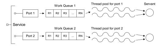
Figure 5: Outline of the Per-Port Threading Model
