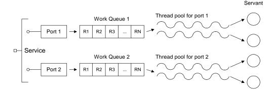
Figure 6: Outline of the PerThread Threading Model
