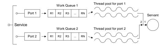
Figure 4: Outline of the Serialized Threading Model
