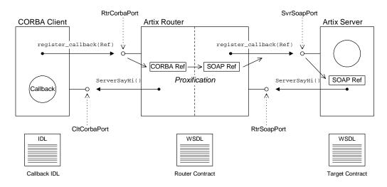
Figure 14: Overview of a Callback Routing Scenario
